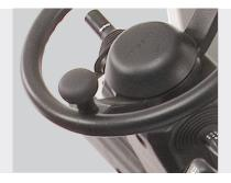
**Steering Wheel Spinner Knob** Provides easier operator control and handling.
